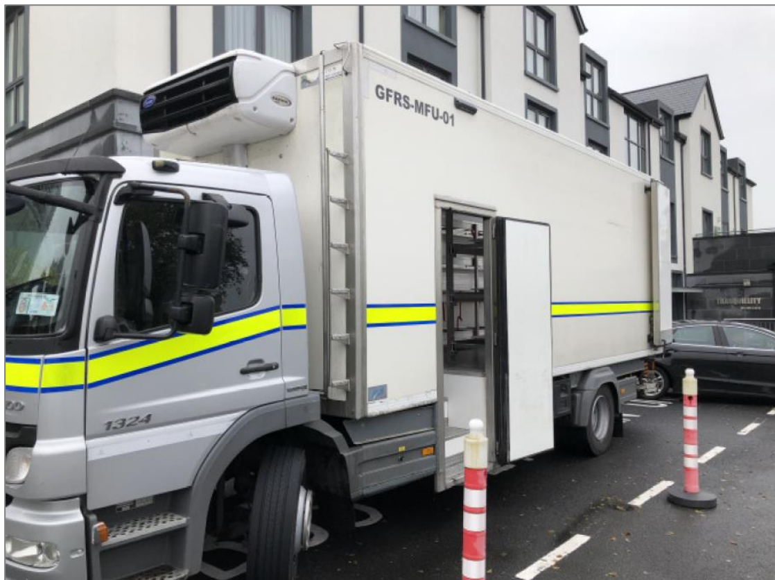
Figure 10: GFRS MFU-01 Refrigerated Body Holding Truck
