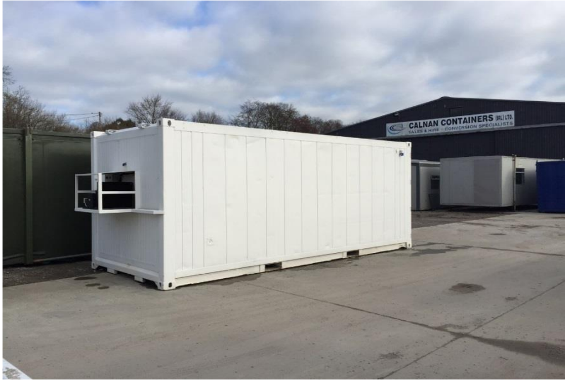
Figure 13: Refrigerated Multiple Fatality Storage Container Unit
